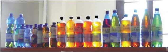
These improper oil sample bottles are real-life examples of what a laboratory may receive.
