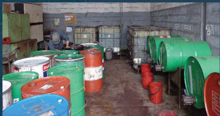
Lubricants were poorly handled, and funnels and buckets were often used.
