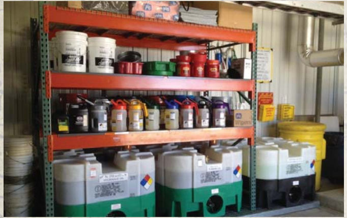
Great River Energy's lube room transformation resulted in the consolidation of oils and lessened the chances of cross-contamination.
