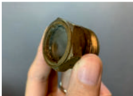
Figure 5: A typical OEM bullseye sight glass.
