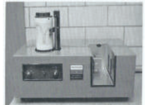
Figure 5: Early table model of an infrared spectrometer. (Ref. Lubrication V.55, Texaco)
