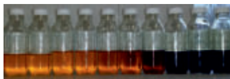
Figure 3: States of degraded oil.
