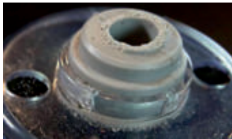
Figure 5: Breather with damaged threading.
