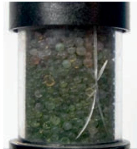
Figure 6: A cracked breather casing.
