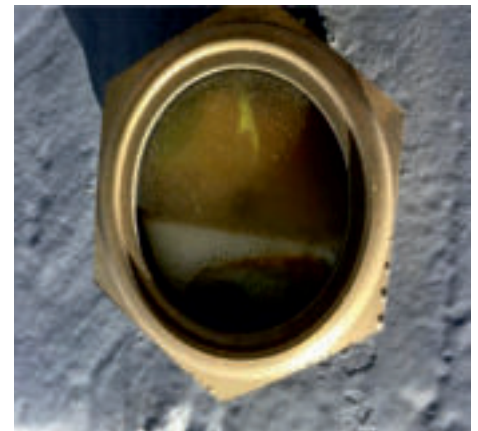
Figure 10: Foamy oil visible through a sight glass.
