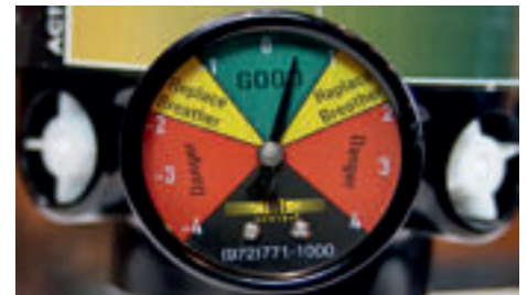
Figure 7: Pressure gauge indicating suitable breather flow.
