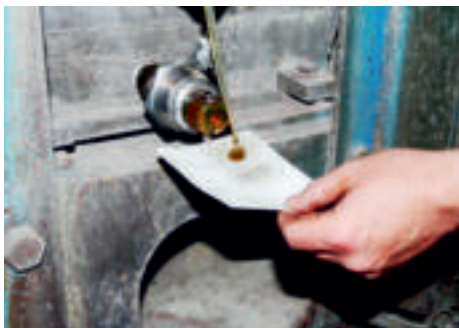
Figure 1: Blotter spot testing: one of the earliest forms of oil analysis.
