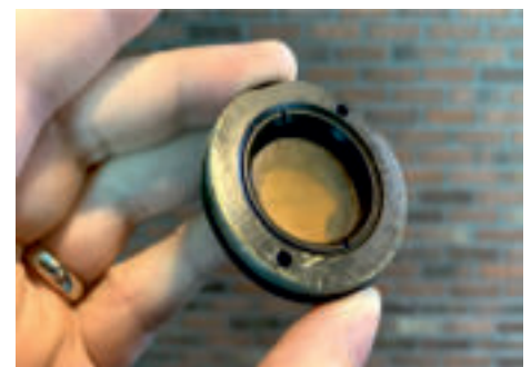
Figure 8: A stained OEM 2D sight glass.
