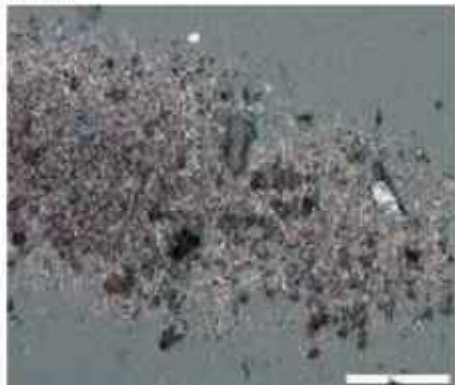
Figure 4. Analytical Ferrogram Showing Corrosive Wear, Abrasives, Lead/Tin Alloy
