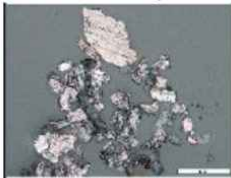
Figure 3. Analytical Ferrogram Showing Ferrous Sliding Wear, Lead/Tin Sliding Wear
