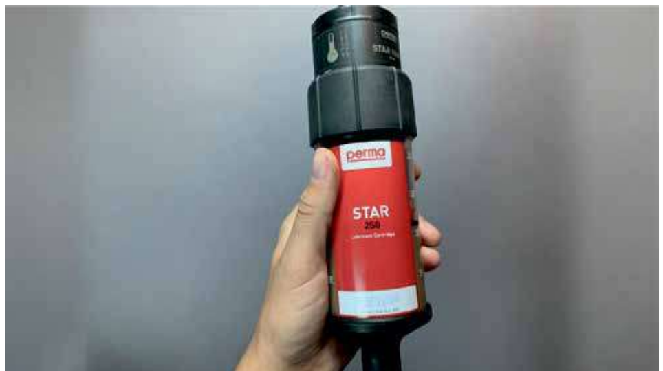
Figure 2: An electromechanical single-point lubricator.
