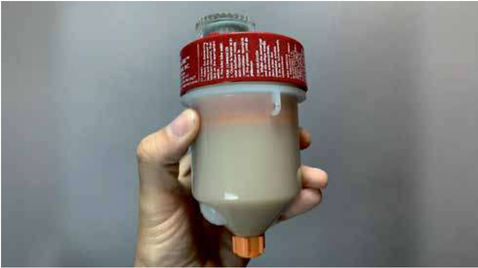
Figure 3: An electromechanical single-point lubricator.
