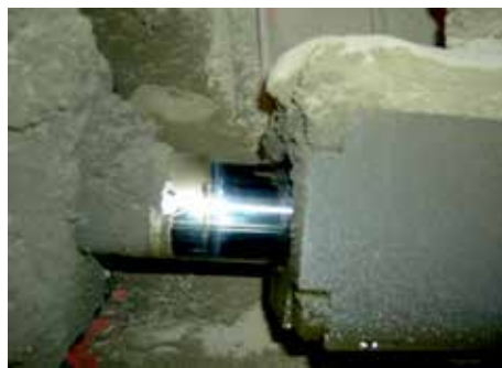
Figure 5. A high percentage of hydraulic system-particle ingress comes into play with the cylinder wiper seal. When looking at this, it is easy to imagine the liquid sandpaper in your oil. Image courtesy of M. Williamson.
