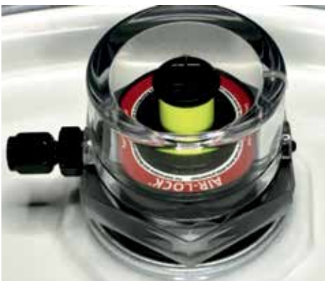
Figure 4. Oil drums breathe in dirt and moisture by thermal siphoning due to routine changes in ambient air temperature. When ambient air cools, air, moisture, and particles can be siphoned into the drum's headspace. Over time, contamination keeps building up in the oil. This device, sold by Luneta, enables quick inspection of this siphoning action so that swift corrective measures can be taken.
