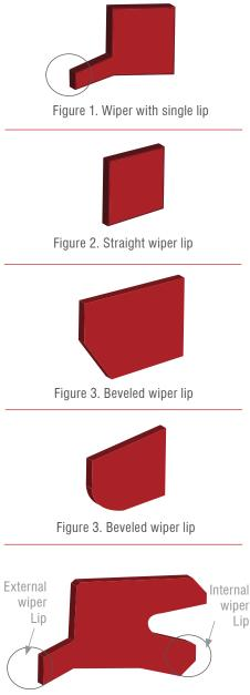
Figure 5. Wiper with double or redundant seal lips
