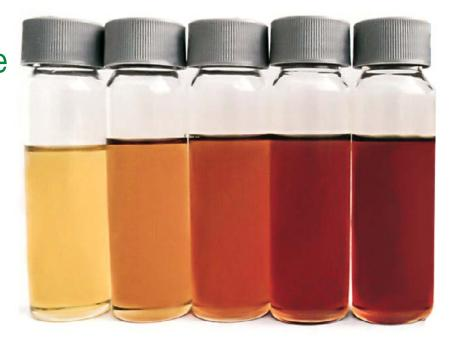
Color can be used as an indicator of oil health, and in many cases it is a reliable field indicator. However, color alone cannot tell the whole story of the oil's condition. For a complete understanding of oil condition, it is important to use an appropriate test slate.
