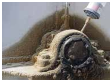
Figure 2. Notice how far oil from purged grease travels along the base and case wall.
