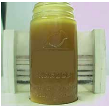
Fig. 4: Turbidity of a mineral oil-based gear oil due to the introduction of a polyglycol
