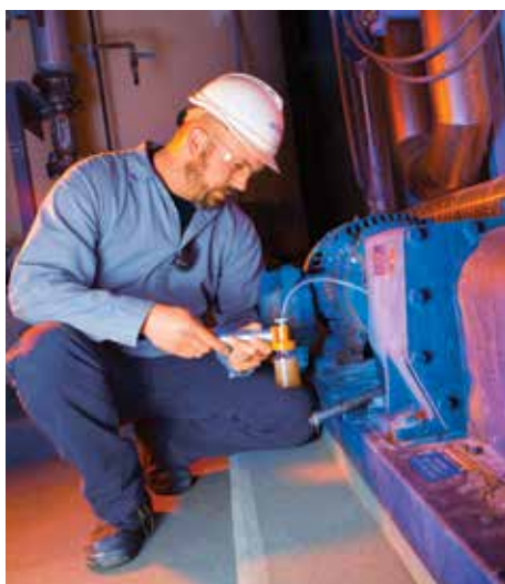
Figure 1: Oil sampling on in-line gearbox.
