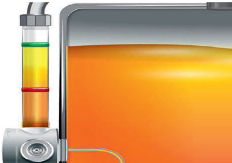
Figure 7: An equilibrium between the lubricant in the machine and the lubricant in the sight glass.
