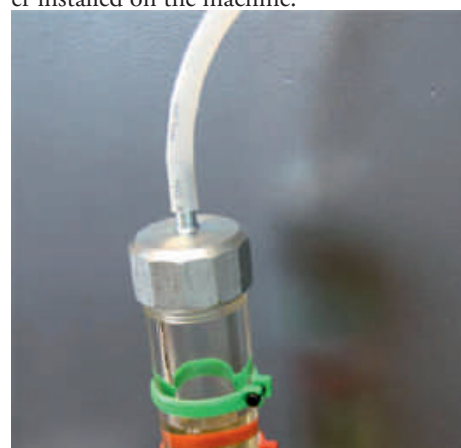
Figure 5: A columnar level gauge with a pipe leading to the machine's headspace.
