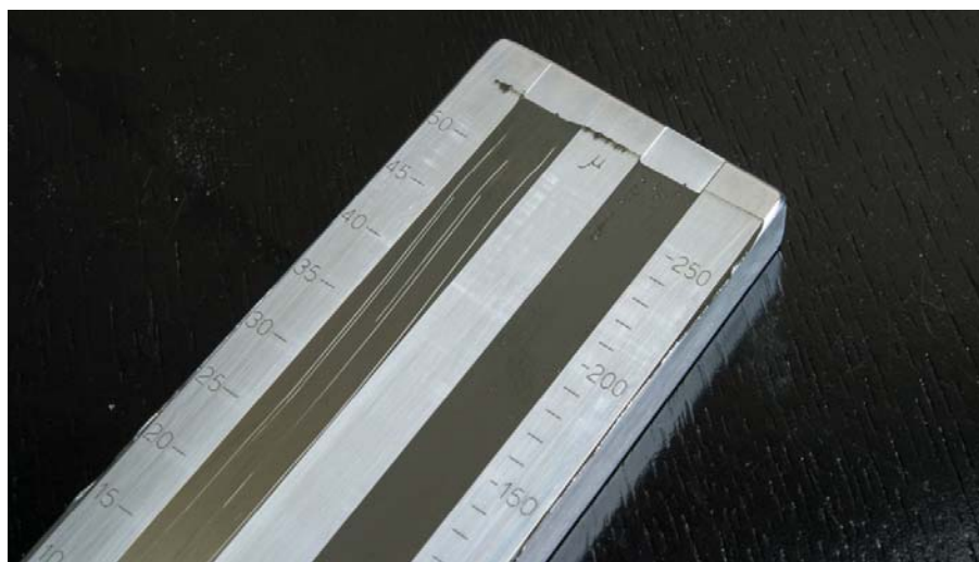
Skid marks left in used grease indicate hard contaminants.
