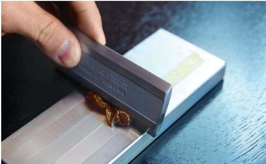
The wiper is pulled down the length of the block with even pressure.
