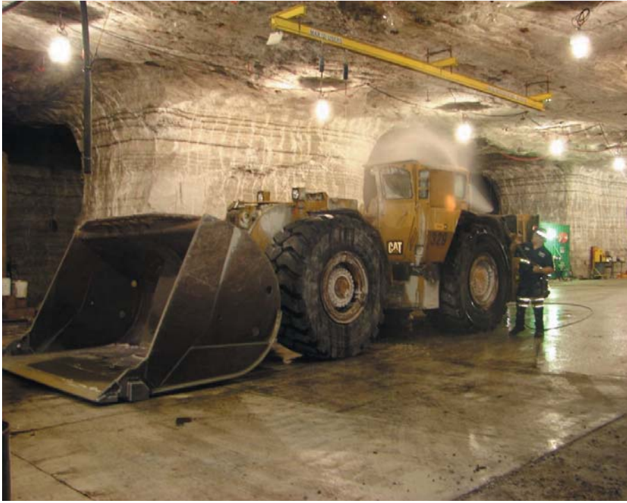
When mobile equipment is scheduled for a PM, it is brought to the new PM facility, where it is first washed and then moved 80 feet for lubrication servicing. PM inspections are then conducted on the clean equipment.
