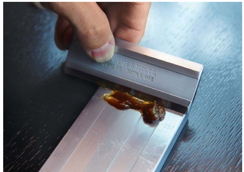
The wiper blade is used to wipe the sample down the block.
