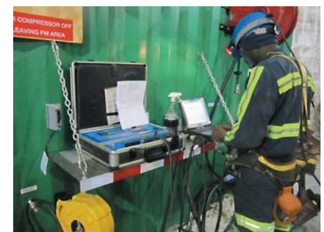
In addition to oil analysis, Cargill also conducts diesel exhaust emission testing to determine engine health.
