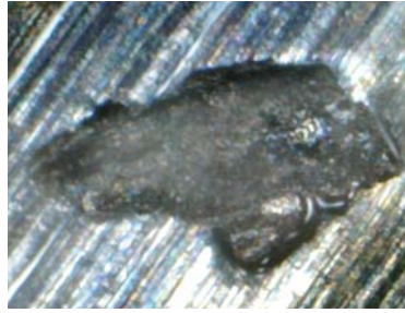
This magnified sample particle appears to be a metal chunk possibly caused by overloading and poor lubrication.
