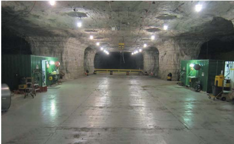
Combined employee ideas culminated in the creation of a new PM facility, which featured all the necessities for oil storage, pumping and filtration.
