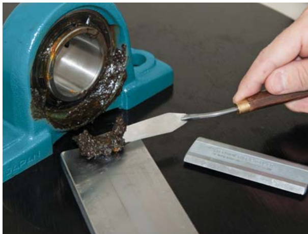
Freshly purged grease should be collected and analyzed for wear debris and contaminants.
