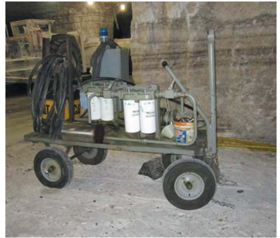
A portable kidney-loop filtration unit was designed to meet the needs of the mining operation.
